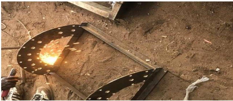
Figure 12: Horizontal Frame Component under production
